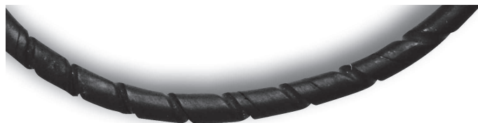
Fig. 9.10 Twisted O-ring with spiral marking
