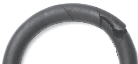
Fig. 9.11 Twisted O-ring with spiral cuts in surface
