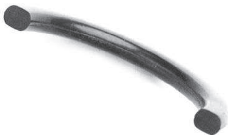
Fig. 9.9 Characteristic compression set. High deformation
