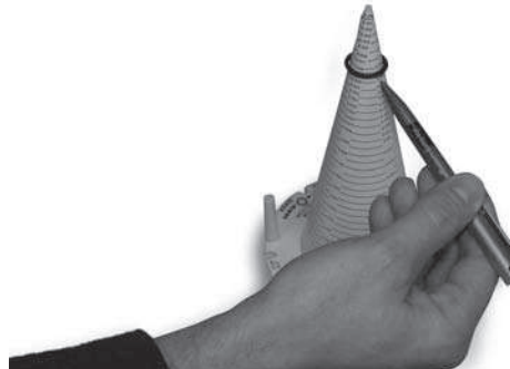
Identification of the 2-xxx size number with the measuring cone
