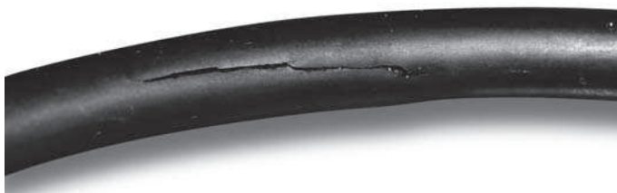
Fig. 9.12 O-ring damaged by explosive decompression
